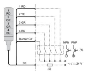
(1) "ON" for lighting and/or applying continuous sound. (2) Fuse (rated current: 0.5 A)
